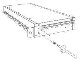
2. From the rear of the cabinet slide the KVM Switch along the rails, until it reaches the console and the thumb screws are aligned to the rear of the cabinet
