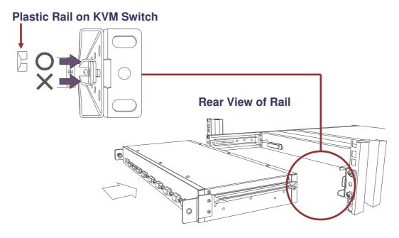
3. Tighten the Thumb Screws of Bracket A, at each side, to fix the position of the KVM Switch and complete the installation
